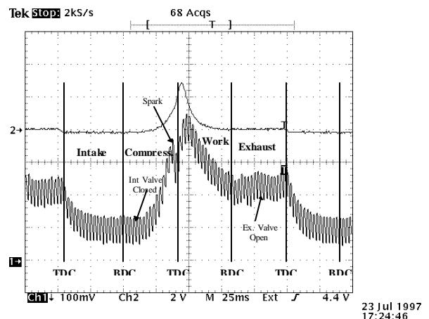
**Figure 6.** A sample of simultaneously obtained cylinder pressure (upper curve) and breakdown voltage (lower curve). Conditions: idle, 680 rpm Breakdown voltage has been inverted in order to highlight its correlation with the cylinder pressure
