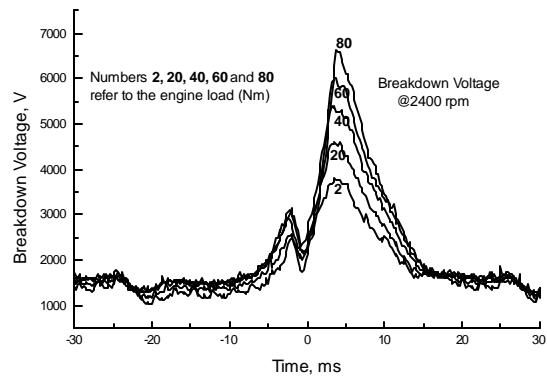
**Figure 8.** Breakdown voltage at 2400 rpm, different loads.
