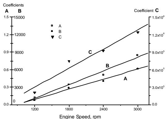
**Figure 10.** The polynomial coefficients are linear functions of engine speed.
