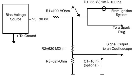
**Figure 1.** Schematic diagram of the measurement circuit. An additional diode can be installed in the line marked "A"
