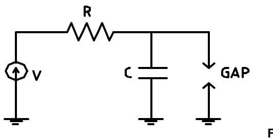
**Figure 2.** A self-oscillating circuit.
