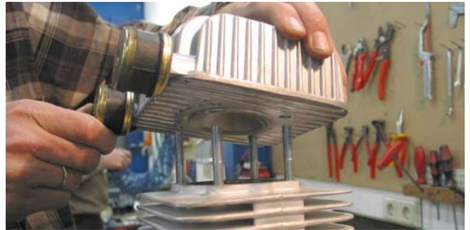
After removing the cylinder you can see the piston. Before you pull out the gudgeon pin remove the safety rings on both sides. Than press out the gudgeon pin.
