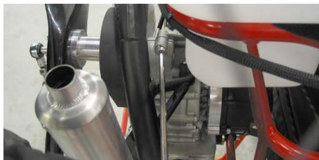
Inside the propellerhub is an allan key-screw. Turn this with the 12 mm allan key until the tension is reached.
