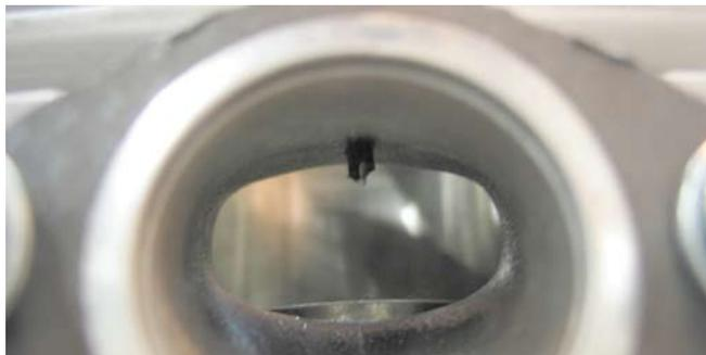
To mount the cylinder you have to press the two pistonrings into the notch.
