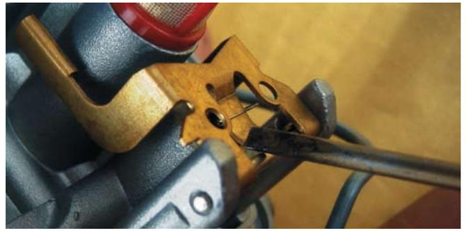
If you hold the carb up side down, the swimmerforc is not parallel to the carburettorcase. If the carb overflow while using the motor the forc should look a little bit more upward.
