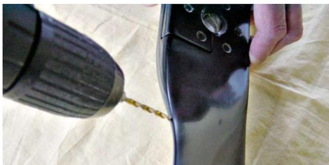
Then fill only as much resin into this hole until the propeller does not want to turn to one side only.
