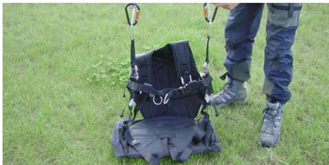
The harness is secured via 3 springlocks; tow legs spring and one breast spring lock. It has two adjustments possibilities. One there are the buckles which are fastened onto the front of the seat. At the start these should be pulled on lightly, as to make the climbing into the harness easier at the lift-off. Before landing it is advisable to lower the seat fully, to enable a maximal favourable touch-down position. The leg loop does not need to be pulled too tightly.
