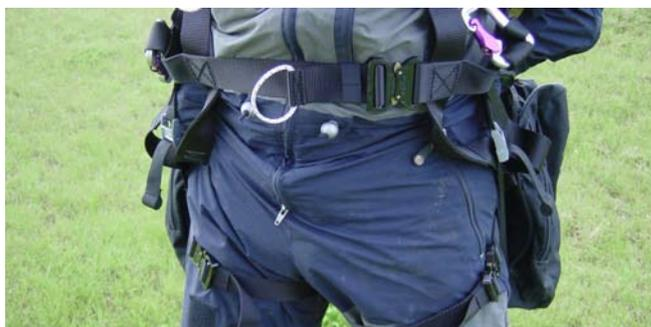
All other adjustment options are regulated while flying. Are the straps pulled right and left, then one sits up straight, are they loose a slight back prone position can be adopted.
