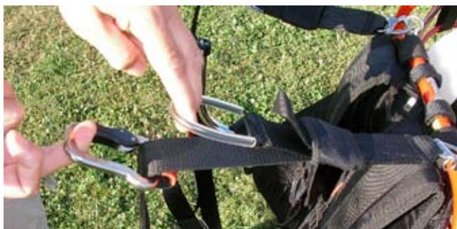
Here you must fix the carringsstraps from harness to the frame.
