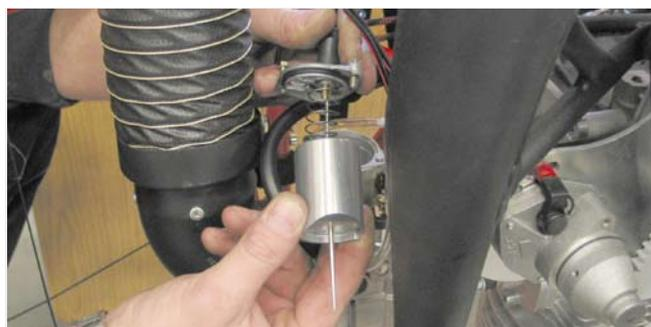
Airbox attachment on carburettor WB 37
