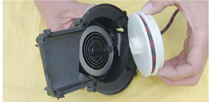
The starter rope can be pulled out of the disc.
