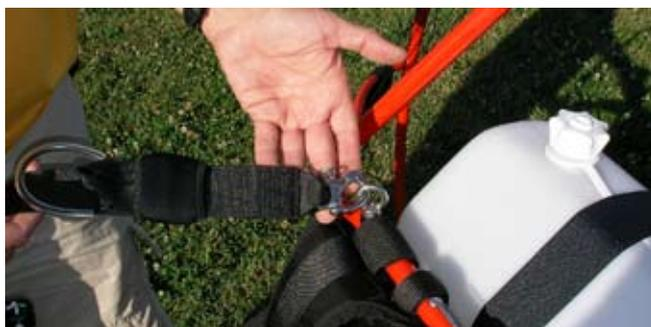
The rear pilotsuspension is adjustable. For basic position pull the loop until the carabiner. Heavy pilots should open and light weight pilots should close the belt.
