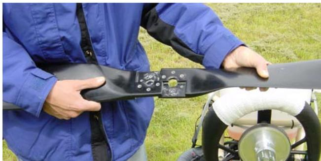
The propeller is fixed onto the hub with 6 screws. Tighten the propeller, use 12 Nm torc.
