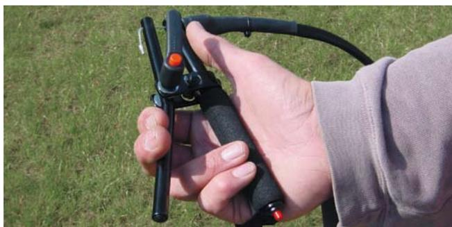
This picture clarifies the handling of the riser and the throttle during the start.
