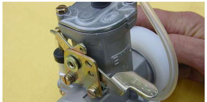
The big screw regulate the idlerunning. Turning right-high rpm. Turning left lower rpm. The idlespeed should round about 240 1/min. The smaller screw is responsible for fuelmixture in idle. Turning right-rich. Turning left-lean
