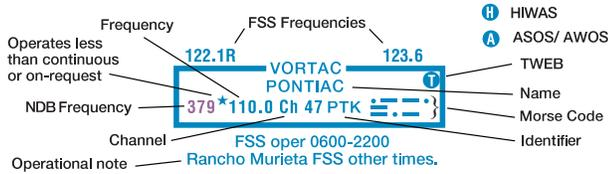
Radio aids to navigation located on an airport depicted by the pattern symbol may not always be shown by the appropriate symbol. A small open circle indicates the NAVAID location when co-located with an airport symbol. The type of radio aid to navigation may be indicated by letter identification; e.g., VOR, VORTAC, or VOR-DME, positioned on and breaking the top line of the identification box.
